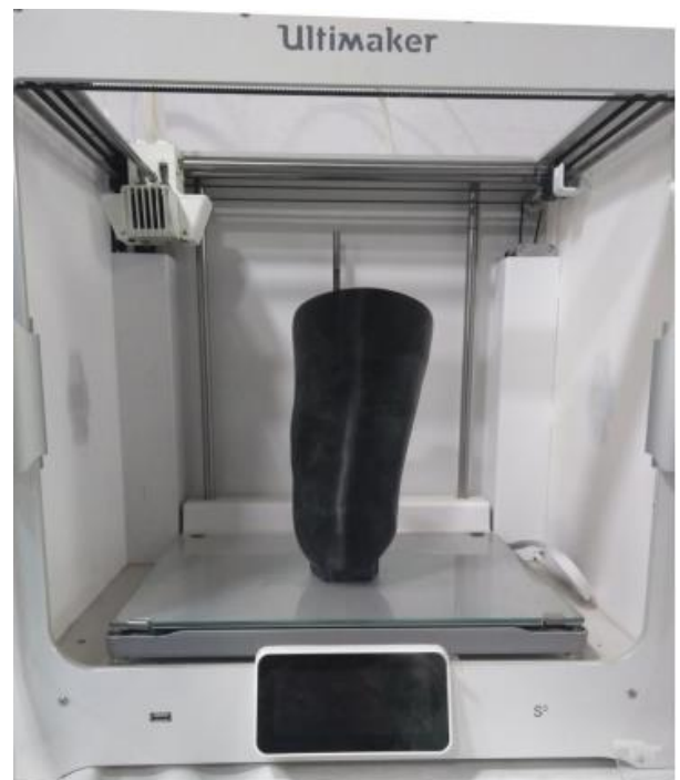
Fig. 10. Socket made using Additive Manufacturing
