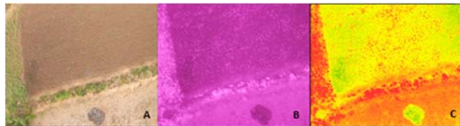
Fig. 8. Normal (A); IR(B) and NDVI (C) image of the field
